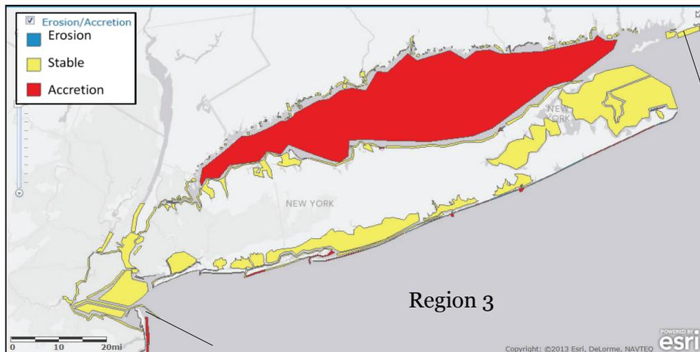
Figure 14. Detail of CRSB for Region 3: from East Rockaway Inlet to Fire Island Inlet, NY.
